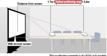
This positioning example is for XGA (4:3) models.
