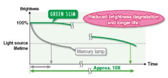
exchanging lamps dramatically, while at the same time maintaining clear, high-quality images over an extended period by reducing the tendency toward degradation of the brightness.
